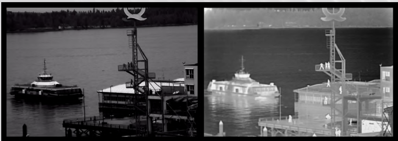
Visible image (on left) shown next to a thermal image (on right) of the same scene. Note the number of people detectable in each image.
