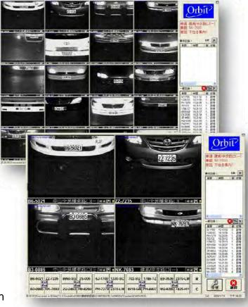
will be notified immediately accompanying the related surveillance video and snapshots. Up to 20 car plates can be simultaneously identified and displayed in one single system, and the maximum detection speed is 120km/h.
