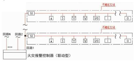
When the bus passes through the fireproof zone, the bus short circuit isolator should be set at the crossing point.
