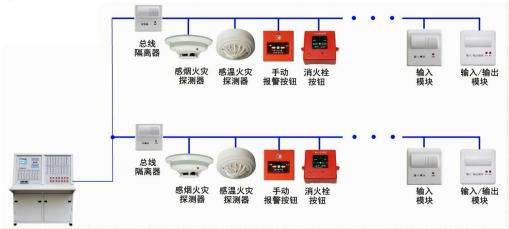
In A ring bus system, the total number of fire detectors, manual fire alarm buttons and modules protected by two bus short isolators should not exceed 32 points.
