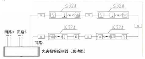
In a tree bus system, the total number of fire detectors, manual fire alarm buttons and modules protected by each bus short circuit isolator should not exceed 32 points. That is, the total number
