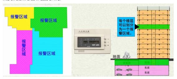
One fire display panel should be set up in each alarm area.
