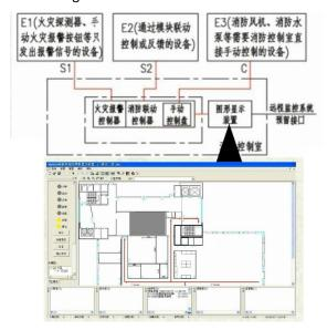
However, the graphical display device cannot reset the controller, set the system, and start and stop the linkage device.
