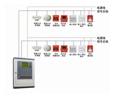
For example, the maximum address point of each loop of the controller is 252. Theoretically, each loop can equip up to 252 address coding devices, corresponding to 252 address points respectively.
