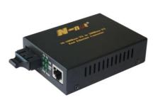
optical networks either by the technology of data link L2 store-and-forward, or by the one of PHY L1 cut-through). It supports transmission in Multi-mode dual fiber or single mode dual fiber.
