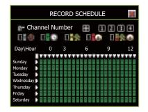
Manage the Schedule for Recording Type The record schedule makes the recording setup more flexible, you can setup the recording type by month, week, day and hour for each channel on-demand.
