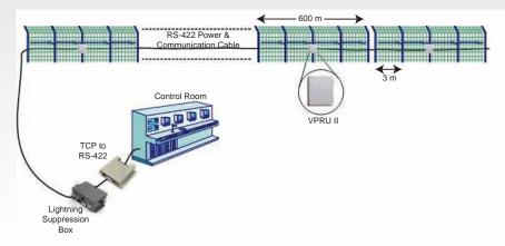
The distance between sensors is defined by the fence structure, normally 2 - 3 meters (6.5 to 10 ft.), or the distance between two supporting posts. This distance sets the resolution of the fine detection algorithm to be 2 - 3 meters (6.5 to 10 ft.).
