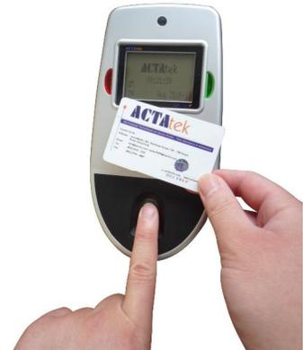
The ACTAtek unit has an embedded web server that is easily accessed by any internet browser from anywhere in the world. By simply connecting an Ethernet cable and powering up the device an IP address can be entered using the keyboard—access is now available. SC Magazine goes on to say *"To setup the device, all we had to do was give it an IP address on our test network via the keypad and we were up and running"*.
