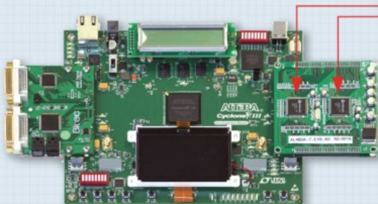
AL460A-7-EVB-A0 board with Altera Cyclone III FPGA Development Kit and Bitec HSMC DVI Daughter card
