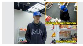
A covert camera installed at the face level can always see the face without being noticed.
