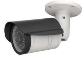
M2387MPE Progressive scan 1/2.9 inch CMOS 2.0M pixels Full HD IR BULLET camera 3.7mm 24IR, TDN, WDR, 0.12 Lux, IP66, POE
