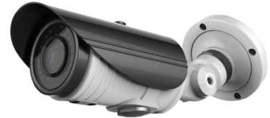
M2389MP Progressive scan 1/2.9 inch CMOS 2.0M pixels Full HD IR BULLET IP camera 3.6~16mm Analog video out (CVBS) Digital PTZ, video crop VANDAL PROOF IR LED, TDN, WDR, 0.12 Lux, POE
