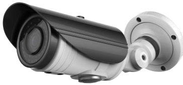
M2389MPE Progressive scan 1/2.9 inch CMOS 2.0M pixels Full HD IR BULLET camera 2.8~12mm 24IR, TDN, WDR, 0.12 Lux, IP66, POE
