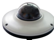
M2361MP Progressive scan 1/2.9 inch CMOS 2.0M pixels Full HD Pancake IP camera 3.7mm Analog video out (CVBS) Digital PTZ, video crop 3Axis Lens mount 18IR, TDN, WDR, 0.12 Lux, POE
