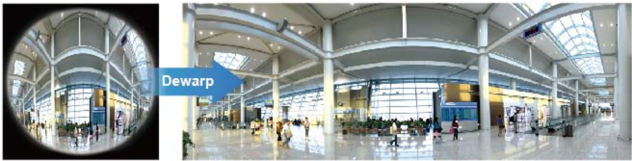
A fisheye lens creates a distorted view of a scene that, once dewarped, provides a powerful surveillance tool that can provide much more detailed coverage than a conventional lens.
