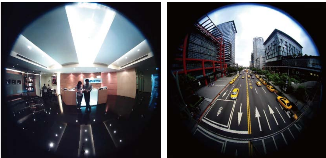
Examples of images captured by a fisheye camera. The resulting image is considered an extreme form of barrel distortion.
