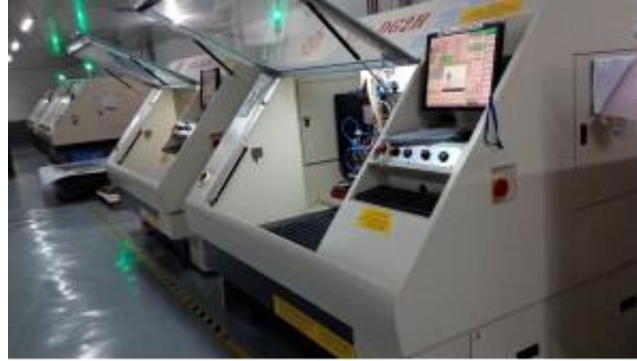
High-speed two-axis drilling machine
