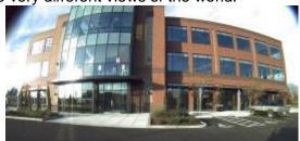
Barrel distortion wide angle lens
