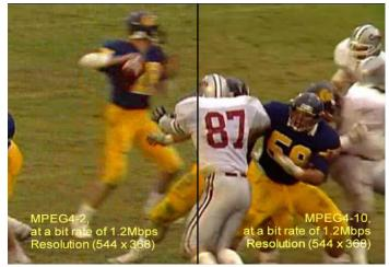
In order to give some practical meaning to the above graphs and numbers, here is a split image from an encoded video sequence<sup>10</sup>. The left side shows the effect of an MPEG-4 Part 2 codec, and the right side the effect of the reference implementation of H.264, at a given bit rate. The improvement is clear enough. Note the blurring and blocking artifacts on the left side.
