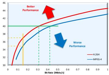
40 dB PSNR. The curves show you that the MPEG-4 encoder performs at 420 kbits/s while the H.264 encoder contains the bit stream to 310 kbit/s. This is about 25 % increase in compression ratio.
