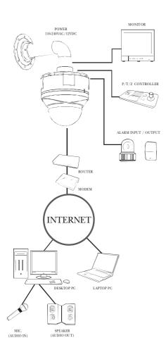
SVD-3020 Network Dome Camera provides advanced solutions for viewing, recording and retrieving video over computer networks, including the Internet. SVD-3020 dome camera delivers superior quality MPEG 4 video steam(at the speed of 30 frames per second) as well as JPEG.
