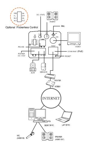
The Intelligent Network Camera SVC-3030 provides advanced solutions for viewing, recording and retrieving video over computer networks, including the Internet. SVC-3030 provides dual video codec. It generates high quality MPEG-4 video stream as well as JPEG which offers more various applications to users.
