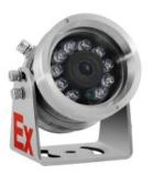
Model: SGC-EX-MS700 Certificate of Conformity (1) Marking: ATEX / Exd II CT6 / DIP A20 TA,T6 (2) Cer. No.: CNEx11.0277 Mechanical features (1) Material: 304 Stainless steel [316 optional] (2) Surface treatment : Fluorine-carbon spray processing (3) Ingress Protection: IP68
